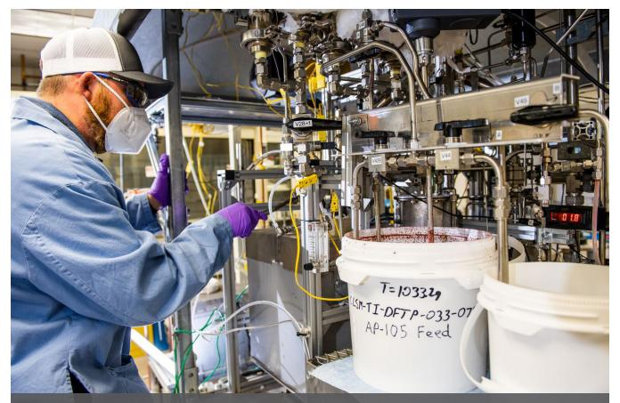
One of the many ways PNNL researchers support Hanford Site operations is by running simulated tank waste in a Continuous Laboratory Scale Melter in the Wasteform Development Laboratory—prior to running actual Hanford tank waste through similar equipment in the Radiochemical Processing Laboratory. Pictured on the cover is the viewport where researchers observe the cold cap, which is the slurry that floats on the molten glass before it has fully reacted. Photo by Andrea Starr | PNNL
